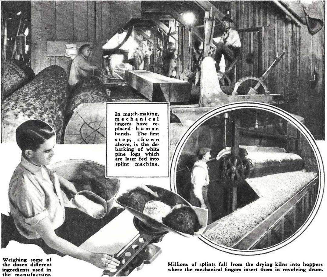
In match-making, mechanical fingers have replaced human hands. The first step, shown above, is the de-barking of white pine logs which are later fed into splint machine.
