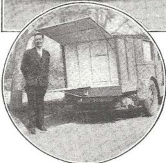
Here is an unusual trailer built by W. H. Shepard of Spokane, Wash., who received third prize of \$2.00 this month. The trailer is made from an Essex body cut off ahead of the rear door. It was relined and addition put on the rear for cupboard and closet space. It contains a bed, made up at all times, sink, 30 gals. of running water under 60 lb. pressure, ice box, gas stove, electric lights, air brakes. Above—A side view. Left—Shepard standing at the rear of his trailer.
