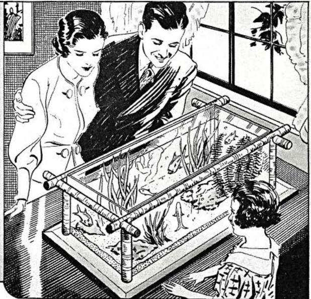
Plate glass from automobile windows is ideal for an aquarium. Straight cuts are necessary, especially at the corners where a water-tight joint is required. Aquarium cement will fill up the smaller cracks. Bottom glass is set in last. Cut all pieces to dimensions given, set up on baseboard, trace around inside and outside edges, then cut the  $\frac{1}{4}$ " deep grooves into which glass will fit, using a chisel or circular saw for routing.
