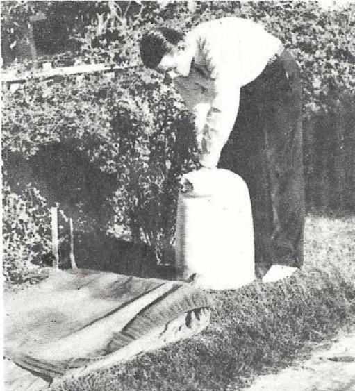
Three strokes of this novel canvas bag air pump are sufficient to inflate an air mattress. The bag also can be used to hold water for a shower bath or as a duffle bag.
