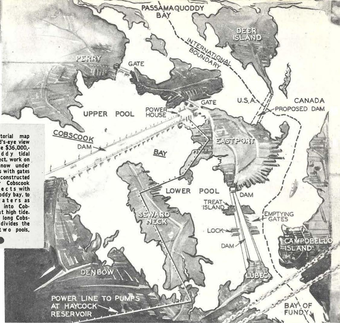
This pictorial map gives a bird's-eye view of the entire \$36,000,000 Quoddy tidal power project, work on which is now under way. Dams with gates are being constructed wherever Cobscook bay connects with Passamaquoddy bay, to impound waters as they rush into Cobscook bay at high tide. The 4-mile long Cobscook dam divides the bay into two pools.
