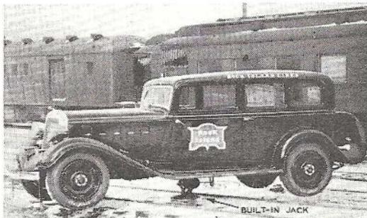
This built-in jack, mounted directly under the center of gravity, serves as a convenient turntable for this rail car. It is the only type of jack which can lift the entire car at once.
