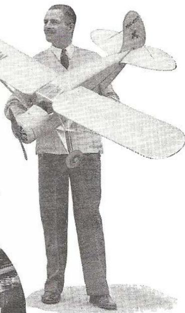
The dangers and expense of filming mid-air plane crashes led Reginald Denny to design and build the model plane with which he is shown above. It has a wing spread of 71 inches and a 1/5 h.p. motor. Two such models can be adjusted to crash several hundred feet in the air, saving thousands of dollars.
