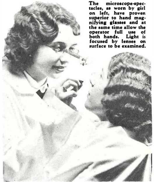
The microscope-spectacles, as worn by girl on left, have proven superior to hand magnifying glasses and at the same time allow the operator full use of both hands. Light is focused by lenses on surface to be examined.
