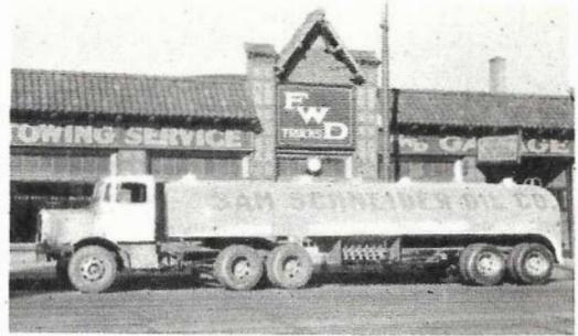
As long as the average freight car, this streamlined gasoline truck is used to make deliveries in sparsely settled areas. The 18-ton load is distributed evenly over each of the 18 wheels.
