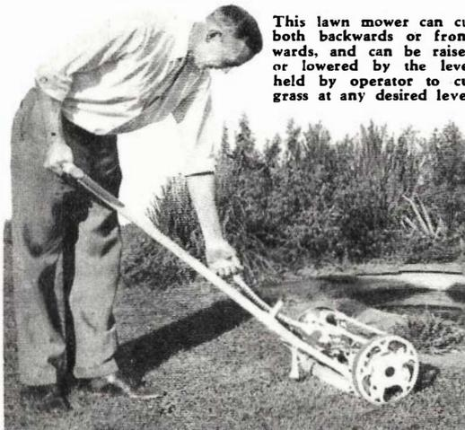
This lawn mower can cut both backwards or forwards, and can be raised or lowered by the lever held by operator to cut grass at any desired level.
